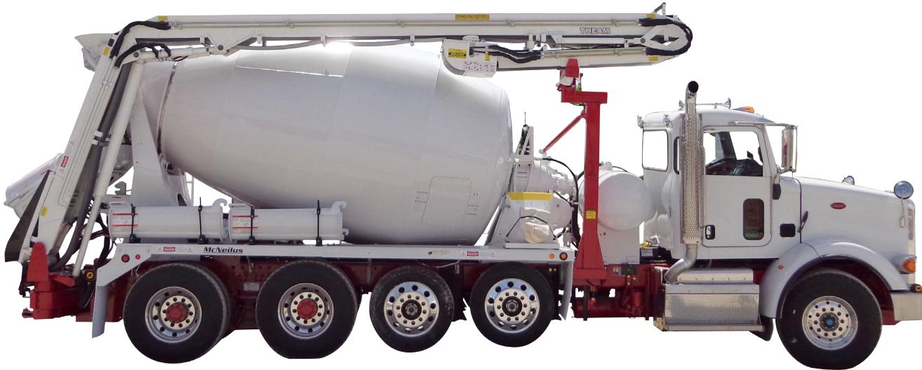
**42A-ALUMINUM** MEET THE LIGHTEST CONVEYOR IN THE LINEUP. This conveyor will accommodate the largest range of “host” trucks. It offers the best payload. It is the good choice for operations facing weight restrictions.
