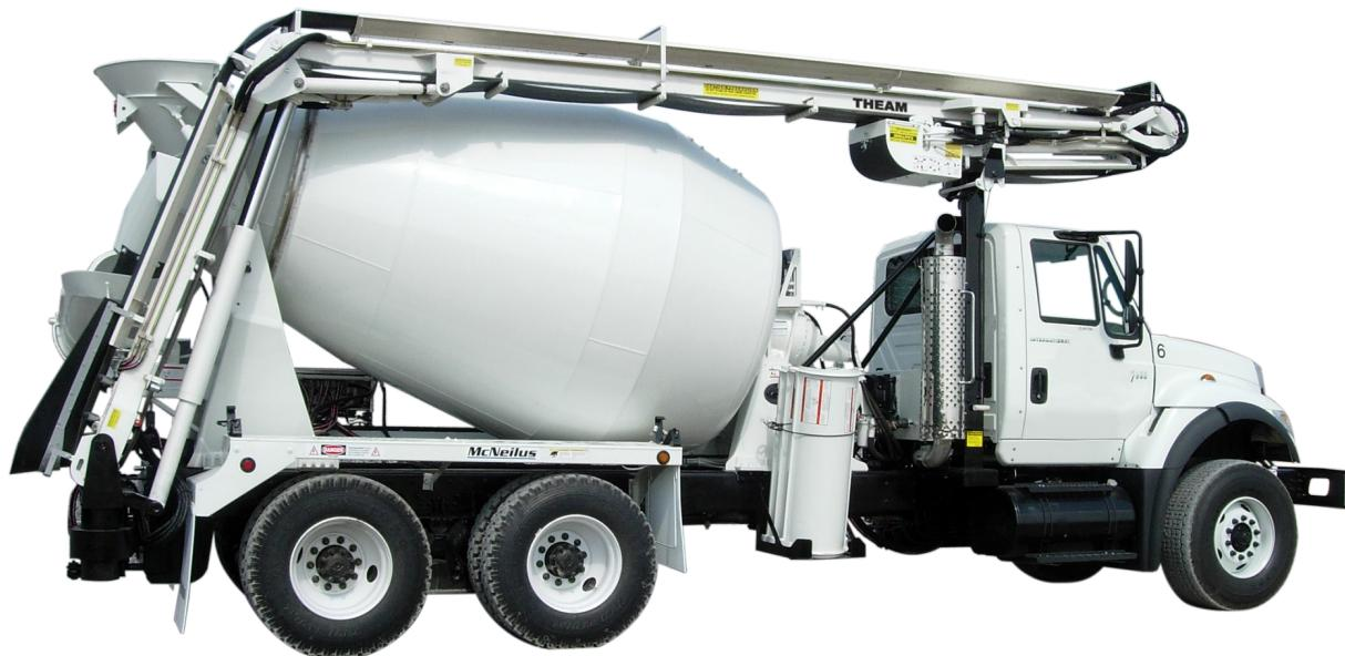
**42S S/L-SLIDER** MEET THE FIRST CROSS-OVER CONVEYOR IN THE LINEUP. This conveyor is a 42S with a twist. We replaced the roller belt support with the 42A's trough design. You get a smooth slide from hopper to hopper.
