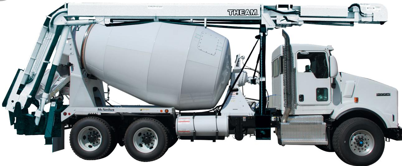
**TLD-DOUBLE TELESCOPIC** MEET THE MOST SERIOUS COMPETITION IN THE LINE UP. This conveyor telescopes on both the tip and middle section giving it the MAXIMUM REACH and the MAXIMUM Telescoping Capacity of any other. It can give a concrete pump a run for its money. That's not the point of any of our conveyors but this model does show teeth. It would be a good choice for the operation that is seasonal, rural or remotely located in places where pumps are few and far between.
