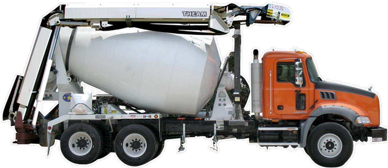
**CROSSVEYOR 30/42** MEET THE SECOND CROSSOVER CONVEYOR IN THE LINE UP. This conveyor introduces a telescoping capacity, 30 – 42 ft. and being free-standing offers mobility around site. This is a good choice for any operation and particularly one in urban environments with sometimes small, limited access to points of pour.
