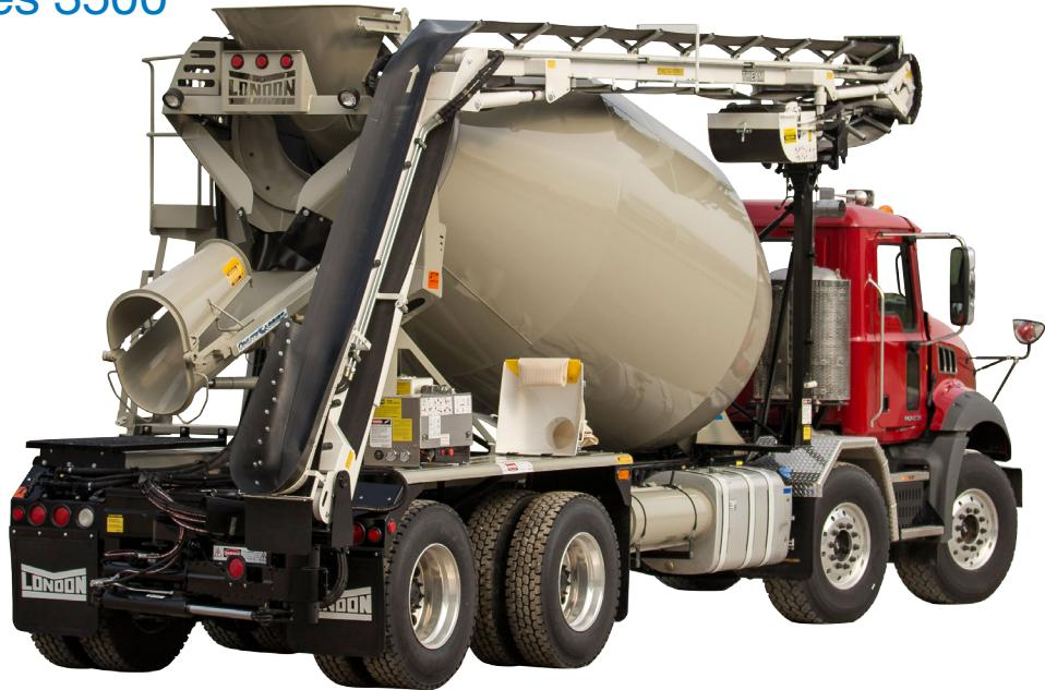
**42-ONTARIO** MEET THE CANADIAN CONFIGURATION IN THE LINE UP. This conveyor is a 42S designed to optimize placing for the wheelbase and twin steering axle trucks common in the region.
